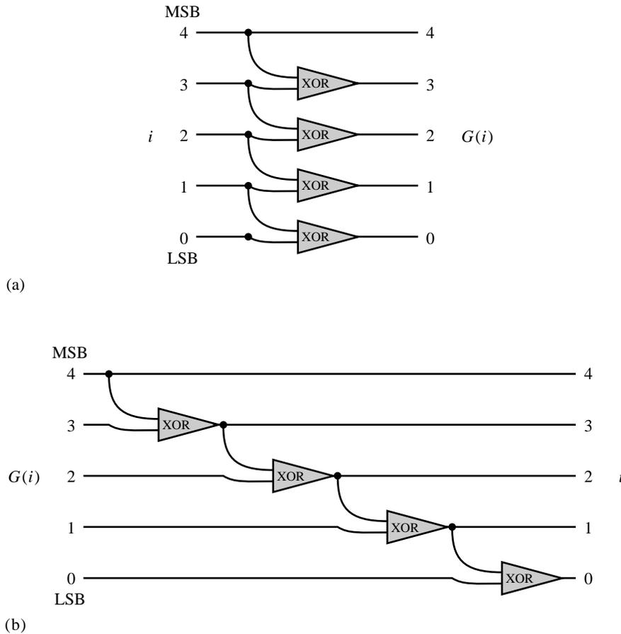
Figure 20.2.1. Single-bit operations for calculating the Gray code  $G(i)$  from  $i$  (a), or the inverse (b). LSB and MSB indicate the least and most significant bits, respectively. XOR denotes exclusive-or.
