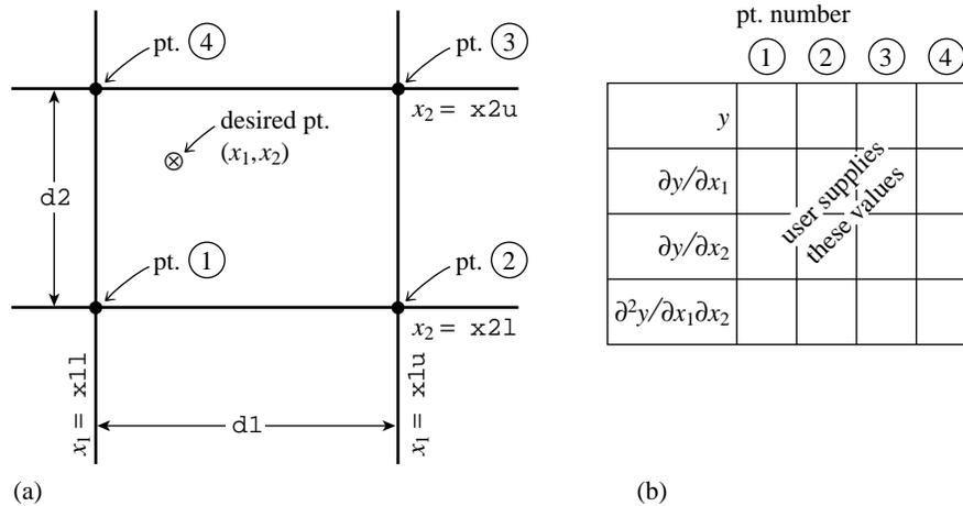
Figure 3.6.1. (a) Labeling of points used in the two-dimensional interpolation routines `bcuint` and `bcucof`. (b) For each of the four points in (a), the user supplies one function value, two first derivatives, and one cross-derivative, a total of 16 numbers.
