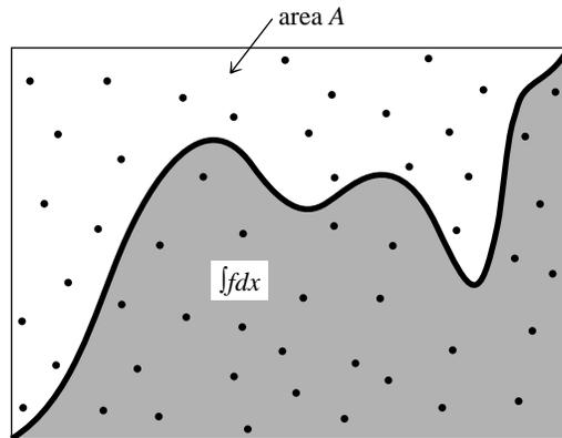
Figure 7.6.1. Monte Carlo integration. Random points are chosen within the area  $A$ . The integral of the function  $f$  is estimated as the area of  $A$  multiplied by the fraction of random points that fall below the curve  $f$ . Refinements on this procedure can improve the accuracy of the method; see text.
